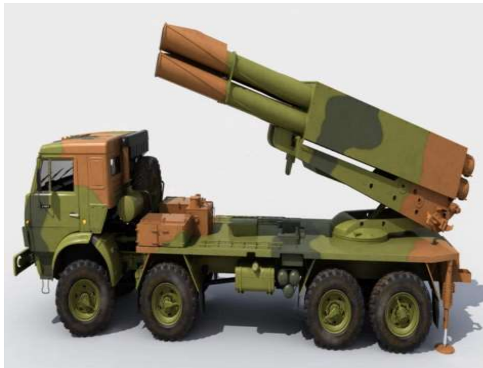
Fabricated components like, Under Frame, Rotating Base Body and Launch Beam Assembly for Rocket Launchers
