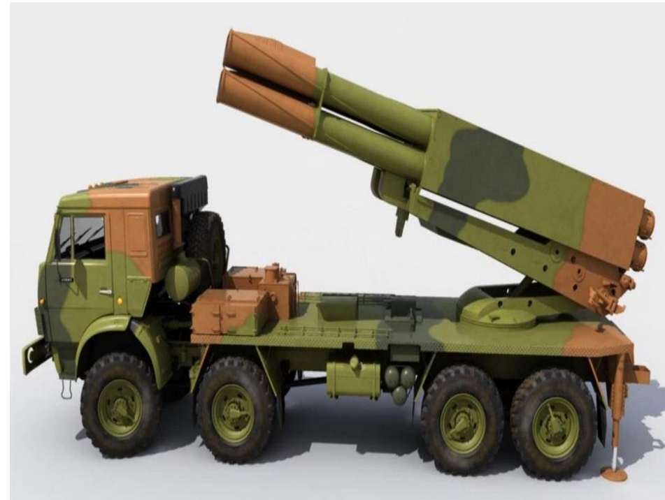
Fabricated components like, Under Frame, Rotating Base Body and Launch Beam Assembly for Rocket Launchers
